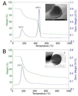
**Figure 3.** (A) TGA thermogram of partially functionalized PE fiber (inset: scanning electron micrograph of pyrolyzed fiber from a partially sulfonated polyethylene). (B) TGA thermogram of fully functionalized PE fiber (inset: scanning electron micrograph of pyrolyzed fiber from a fully sulfonated polyethylene).
